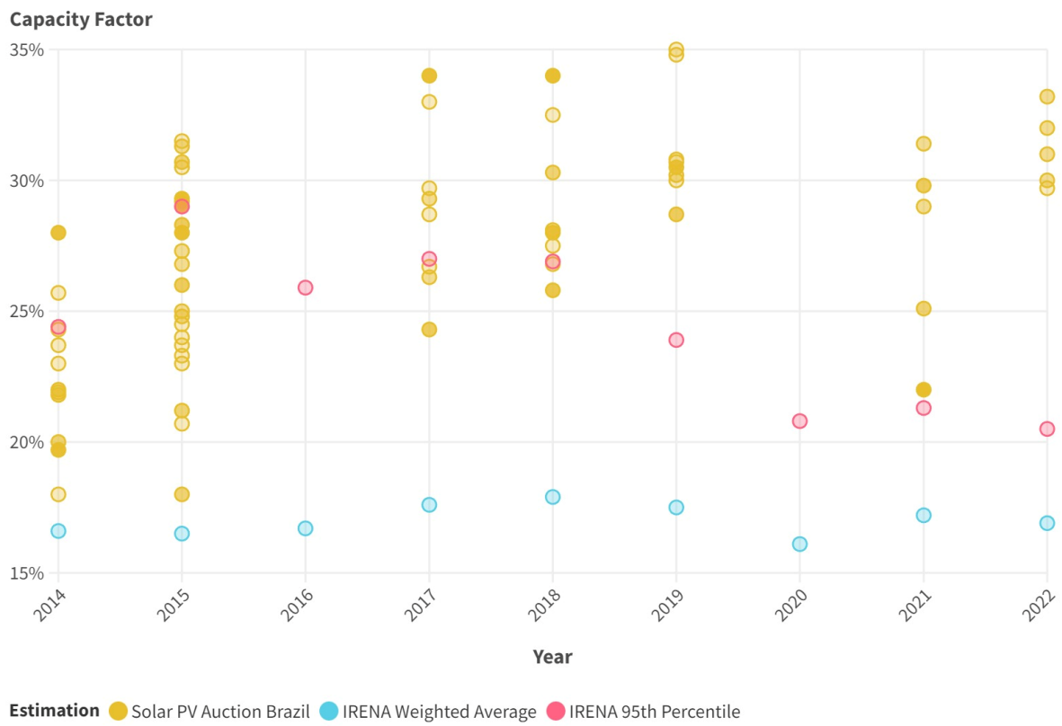
Figure A19. Capacity Factors from Solar PV projects in Brazil. Data sources: CCEE (2024); IRENA (2023)
